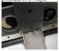
We got rid of the 5/8" spacers so the vertical plate could move forward, away from the pipe. We cut the corners off the bottom edge of the vertical plate so the plate would sneak ahead even more. We (you) may have to flip the bottom Allen screw around so the pipe doesn't hang up on the nut
