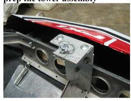
The upper portion of the tower has slotted holes. Raise the upper portion of the tower and semi snug the short Allen screws. Eye ball the Dzus hole and snug that plate. When you begin to install the hood you want the tower parts to yield to the downward pressure of the hood as it is put in place.
